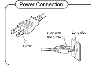
A circle is assigned on one side of the plug of the AC power cable so that better quality sound is reproduced by matching the power supply polarity with another equipment.
