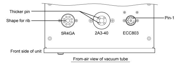
(3) After mounting all vacuum tubes attach the vacuum tube cover.
