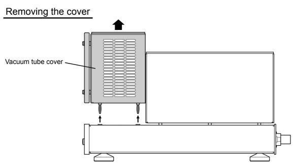
(1) Remove the vacuum tube cover straight up.
