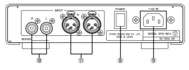
®Power Switch This is the switch that turns the power on/off.
