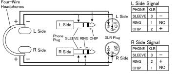
If using four-wire headphones at DUAL MONO, the wiring specifications is as shown above. Check it when purchasing or creating four-wire headphones.
