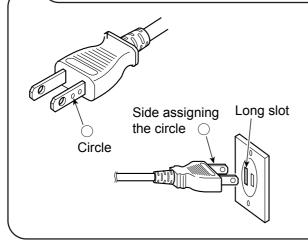
A circle is assigned on the one side of the plug of AC power cable so that better quality sound is reproduced by matching the power supply polarity with other equipment.
